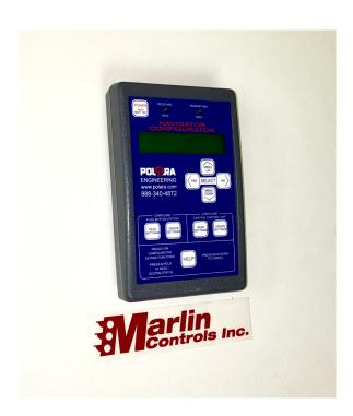
The EZ Configurator (ECONFIG) is a hand held remote used for configuring a Navigator APS Push Button Station. Just stand a few feet in front of a Navigator, point the Configurator at the button, turn it on and select your options. The Configurator communicates via. infrared with the PBS. One Configurator is all you need for maintaining multiple intersections.
