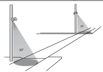
The new SmartWalk XP is part of MS SEDCO's Automated Pedestrian Protection System. This microwave pedestrian presence sensor is designed for curbside, hands free activation of pedestrian signals.
